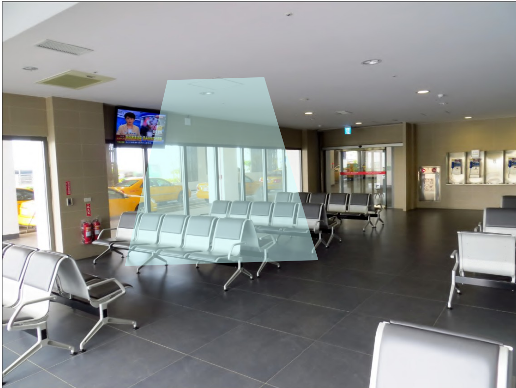
Desired audio zone to cover the seating with the visual range of the TV monitor at an airport waiting area Figure 2
